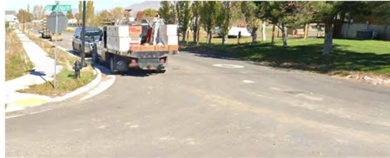
Segment is newly constructed. Access is adequate on South end. The asphalt widths are within the City Code standards except for the last 180 feet on the North end.
